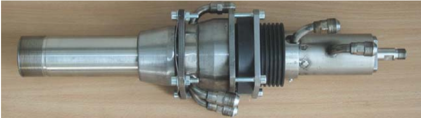
HTT uses plasma arc torches ranging in power from 50 kW to 500 kW to process a wide range of waste products.
